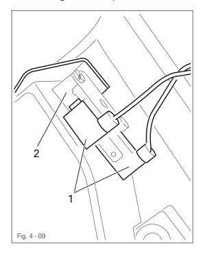
Connect plug 1 of safety switch 2 as shown in Fig. 4 - 09.
