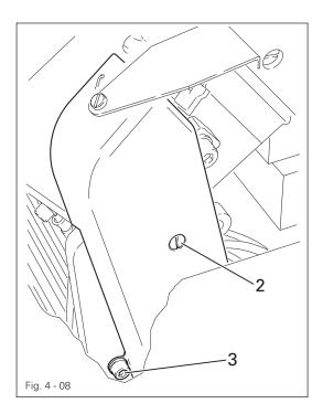
• Attach belt guard 1 with screws 2 and 3.
